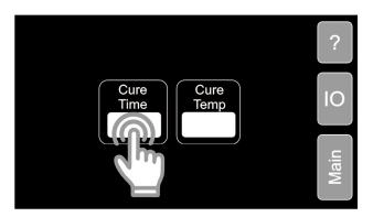
Click the white box under "Cure Time" to input the desired curing time. The unit for input is in seconds. **Value range 30-900 Seconds.**
