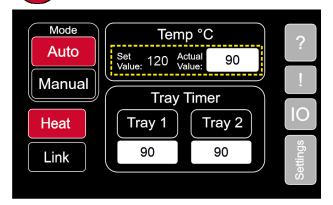
The actual temperature of the oven must reach the set temperature. For example, if the set temp is 120°C you need to wait until the actual value reaches 120°C
