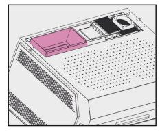
Pull the old filters out and install the new filters (Carbon at the bottom).
