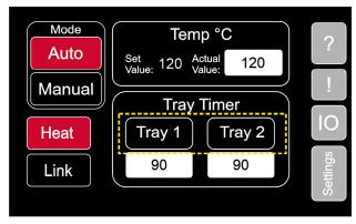
When the countdown for Tray 1 ends, Tray 2 will automatically move into the oven and start curing, with the timer beginning. At this point the media sheet and Tray 1 will have been cured, replace it with a new media sheet on Tray 1, Once tray 2 finishes curing and ejects automatically Tray 1 will move into the oven and start curing. **This process will continue alternately.**
