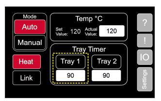
After closing Tray 1, the white box under "Tray 1" on the control panel will start the countdown timer.
