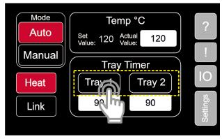
In manual mode after the tray countdown ends it will automatically eject, completing the curing process
