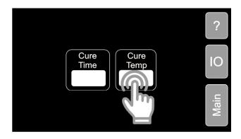
Click the white box under "Cure Temp" to input the desired curing time. The unit for input is in Celsius. **Value range 50-140 C.**
