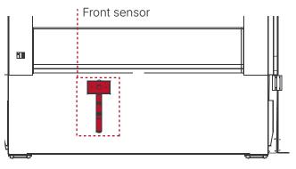
The front sensor has adjustable height levels, allowing users to adjust it to the appropriate position based on their needs.
