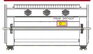
After the transfer film is finished baking, it will exit the oven. The rear sensor is used to detect whether the transfer film has completed baking and emerged from the back.
