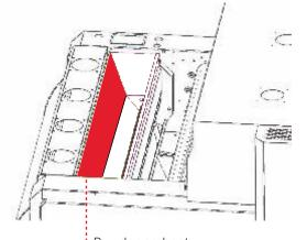
Powder preheat Its purpose is to maintain a high level of dryness for the hot-melt powder inside the box, preventing it from absorbing moisture.
