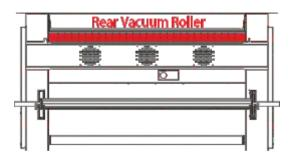
Once the film is detected by the rear sensor, the front vacuum roller will stop suction but continue to transport the film, while the rear vacuum roller will maintain both suction and transport functions.
