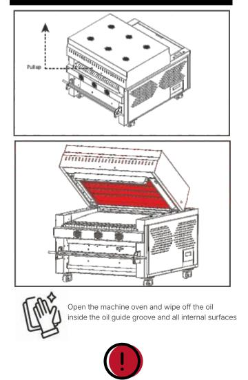
Due to the build up of glycerin/oil which comes from DTF ink it is extremely important that time is taken each day to thoroughly clean excess oil from all surfaces (including inside the lid/hood). The oil residue cannot be fully eradicated due to the oil particles becoming airborne, which forms condensation on various parts of the machine. Failure to clean the surfaces daily can result in oil build up and leakages from various parts of the system and can contribute possibly faults.
