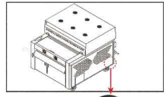
After continuous use please ensure to open bottom valve of the filter to drain the collected oil
