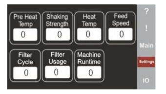
Pre temperature: Operating temperature of the pre-heater
