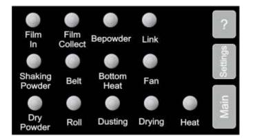
The displayed parameters here correspond to the working status of their respective names and do not support manual adjustment.
