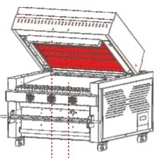
The upper and lower double rows of high-efficiency heating lamps (Lower row is under the feeding belt)
