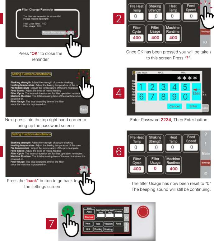
Turn the machine off by the power switch, wait 5 seconds and power the machine back on. The reset has now been completed.
