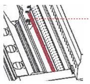
Powder shaking blade Contributing to the uniform distribution of transfer powder through vibrational motion, thereby ensuring high-quality and consistent printing results, located beneath the vacuum roller.
