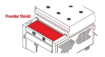
The powder shield's function is to prevent powder from splashing. If it is opened while the machine is running, the powder shaking function will stop. Once it is closed, the powder shaking function will resume.
