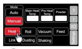
It is recommended to turn on the Heat function for 15 min before starting each work session to enhance the curing effectiveness
